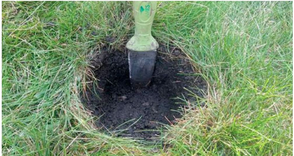
Figure 13: After the 1 hour fill cycle is completed, start tracking the time that is required to drain the test hole completely.
