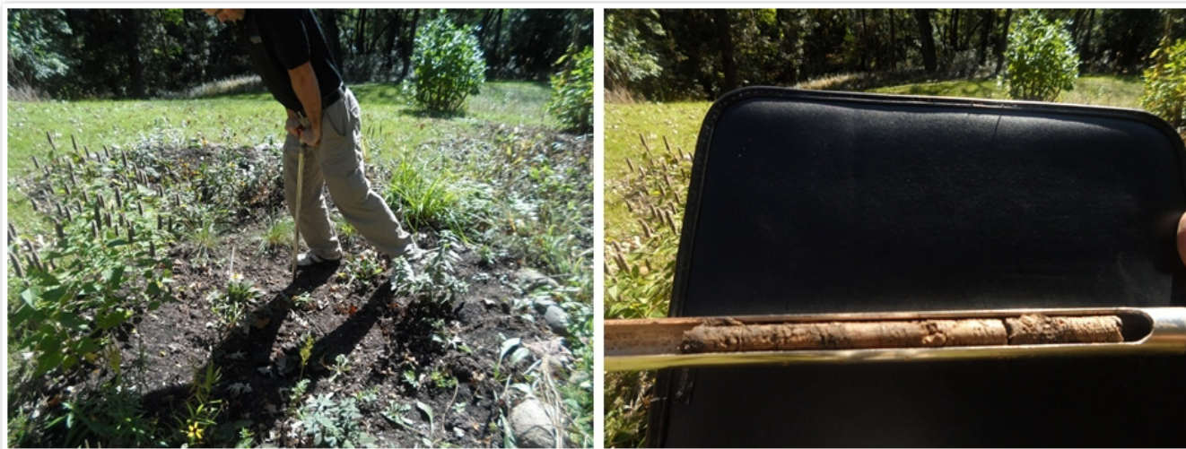
Figure 9: A soil probe can hollow out a core sample 12" at a time.
