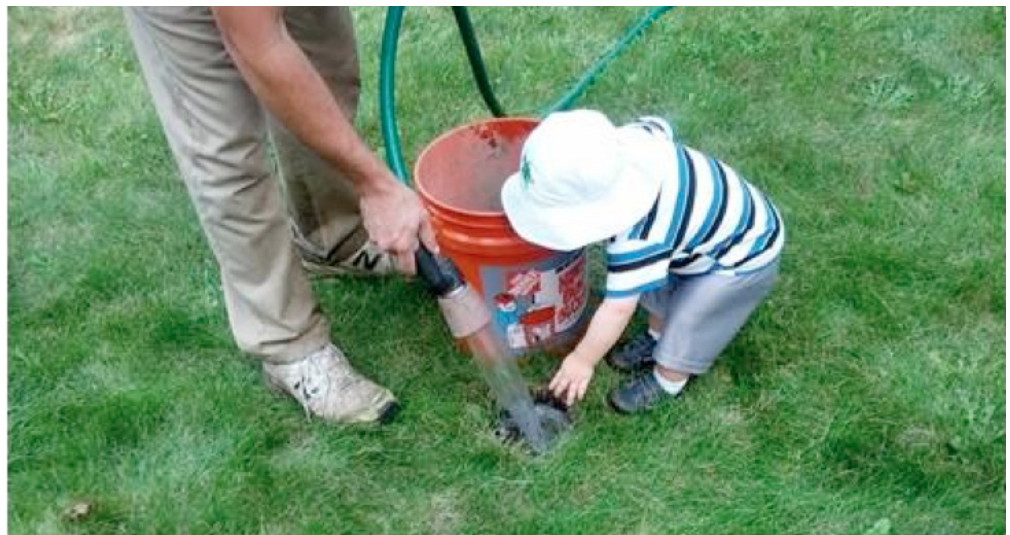
Figure 11: Fill up the test hole with water.
